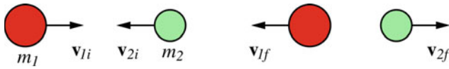
Fig. 5.4 Two particles of masses m_1 and m_2 experiencing an elastic head-on collision
